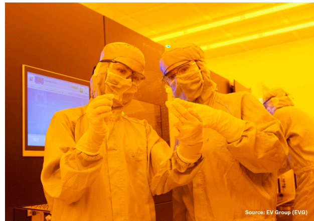
Process engineers at EV Group's NILPhotonics ® Competence Center examine a 200-mm wafer with metalenses replicated using a master manufactured by Toppan Photomask and a nanoimprint lithography (NIL) process from EVG. Source: EV Group.
